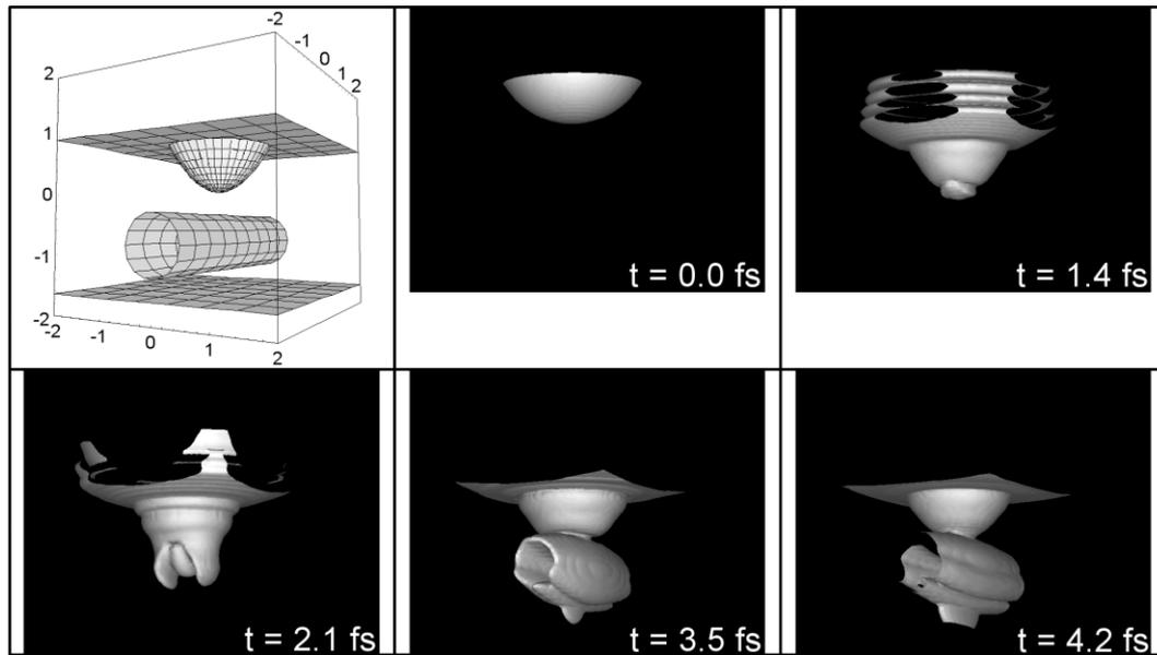
Fig. 1. Time evolution of the probability density of the wave packet approaching the STM junction from the tip bulk and tunnelling through the nanotube into the support. The upper left image is the model system used in the calculation. The labelled box is the presentation box. All dimensions are in nanometres. The subsequent images show snapshots of a constant probability density surface. This surface is clipped at the presentation box boundaries. See the text for details.
