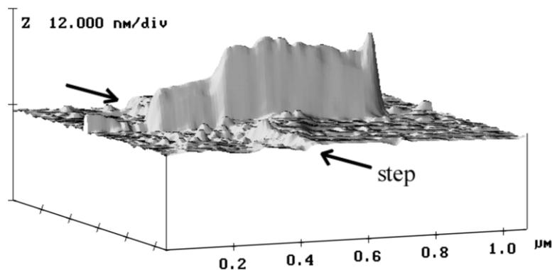
Fig. 2. Constant current 3D STM image of a multi-wall carbon nanotube crossing a step on the HOPG support surface. Note the transition region at the step edge and the gradual decrease of the apparent height of the tube section above the lower terrace.
