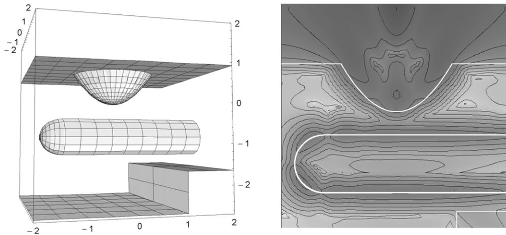
Fig. 3. (a) Model system of a nanotube crossing a HOPG step. (b) Probability density in the plane perpendicular to the support surface and including the tube axis. Contour lines are drawn on logarithmic scale. The thick white lines show the geometrical surface of the tip, nanotube and support.
