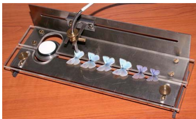
Fig. 2 “Spectroboard” in use. Prepared specimens can be measured rapidly and safely in reproducible conditions. The Avantes fiber optic probe is set perpendicular to the wing surface. In the left upper side is placed the white, diffuse reference standard.
