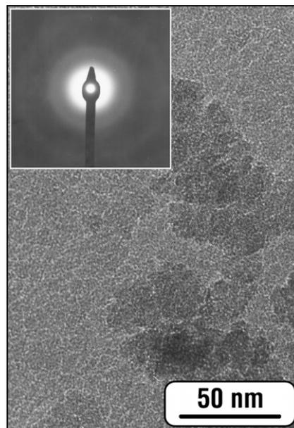
Fig. 2. Plan-view bright-field TEM image of 30-nm-thick  $CN_x$  film deposited at room temperature and  $N_2$  pressure 0.05 mbar.
