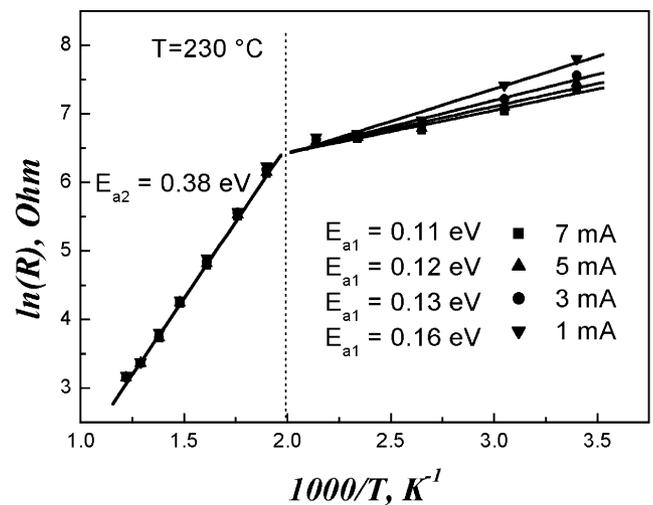
Fig. 9. Temperature dependence of the electrical resistance of 60-nm-thick  $CN_x$  film on Si substrate deposited at a temperature of 800 °C and  $N_2$  pressure of 0.05 mbar.
