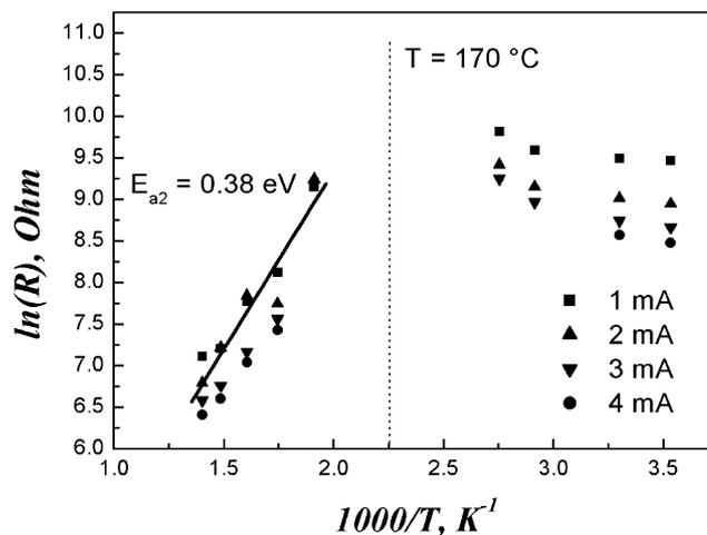
Fig. 7. Temperature dependence of the electrical resistance of 30-nm-thick  $\text{CN}_x$  film on Si substrate deposited at room temperature and  $\text{N}_2$  pressure of 0.05 mbar.
