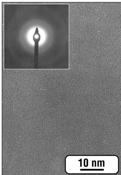
Fig. 1. Plan-view bright-field TEM image of 30-nm-thick C film deposited at room temperature on NaCl substrate.
