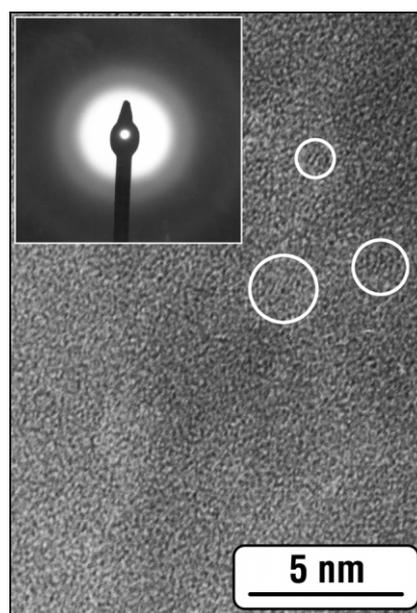
Fig. 3. Plan-view bright-field TEM image of 60-nm-thick  $CN_x$  film deposited at a temperature of 70 °C and  $N_2$  pressure of 0.08 mbar on a Si substrate.
