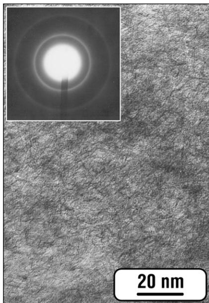
Fig. 4. Plan-view bright-field TEM image of 60-nm-thick  $\text{CN}_x$  film deposited at a temperature of 800 °C and  $\text{N}_2$  pressure of 0.05 mbar on a Si substrate.
