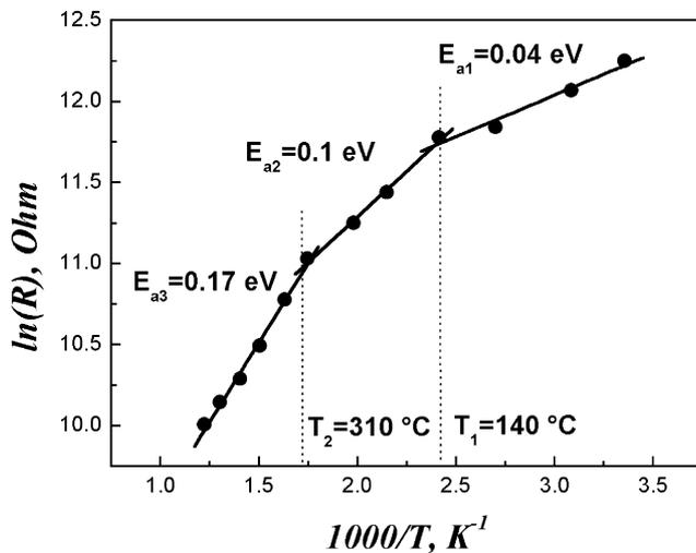
Fig. 8. Temperature dependence of the electrical resistance of 60-nm-thick  $CN_x$  film on Si substrate deposited at a temperature of 70 °C and  $N_2$  pressure of 0.08 mbar.
