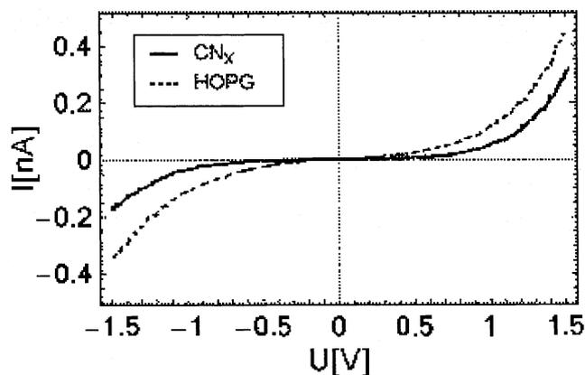
Fig. 5. STS  $I$ – $V$  measurement of the  $\text{CN}_x$  film, compared to HOPG.
