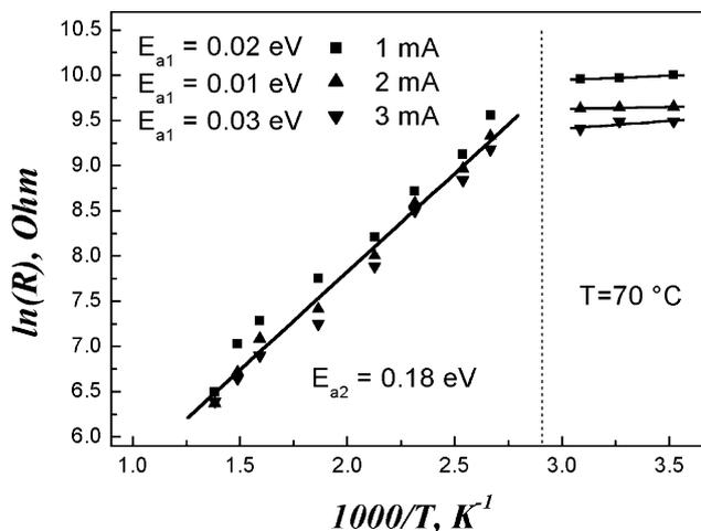
Fig. 6. Temperature dependence of the electrical resistance of 30-nm-thick C film deposited at room temperature.
