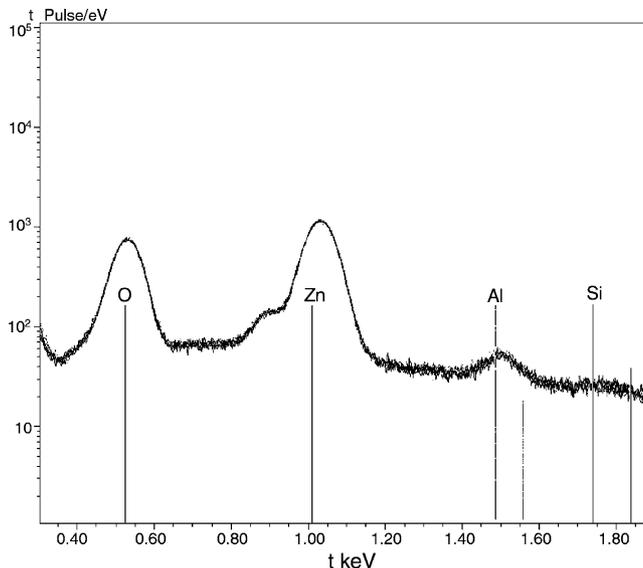
Fig. 3. EDS spectra in 5 analyzed regions of the deposited layer show uniform elemental composition.
