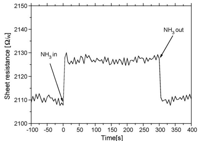
Fig. 6. Typical response of the ZAO resistor to the NH<sub>3</sub> exposure (at 150 °C, 3000 ppm).
