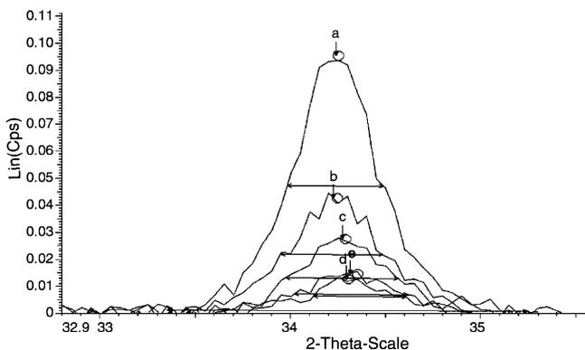
Fig. 5. XRD spectra taken from ‘a’ to ‘e’ places of the sample.
