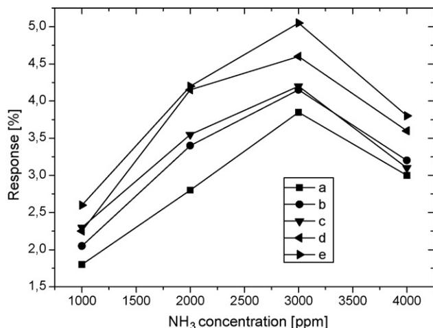
Fig. 7. Sensor response to different NH<sub>3</sub> concentrations affected by the layer morphology.
