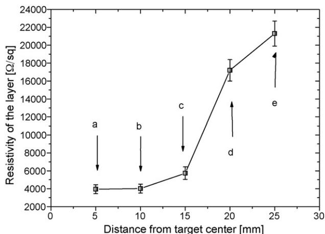
Fig. 2. Sheet resistance vs. distance from the target center (‘a’) in fixed substrate mode (notations ‘a’ to ‘e’ show the sampling locations chosen for analysis.)
