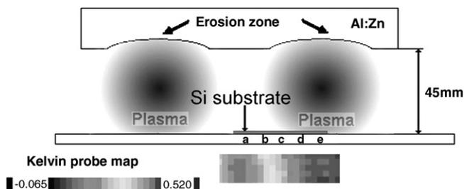
Fig. 1. Schematics of the experimental arrangement and Kelvin probe map of the sample showed at the place of the measurement.
