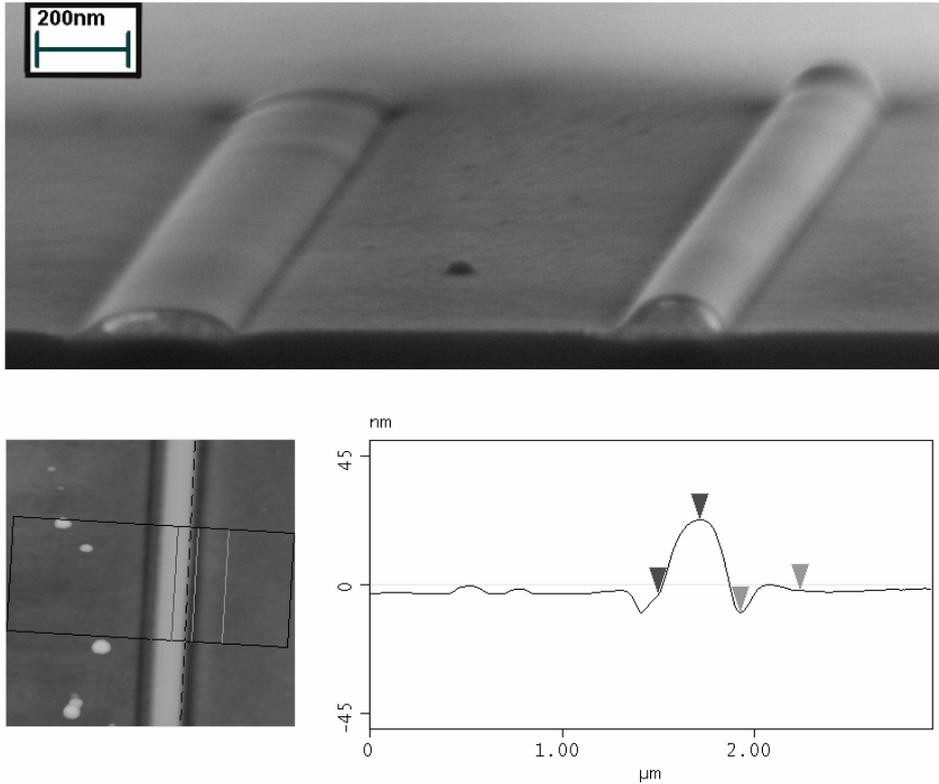
Fig. 5. SEM (a) and AFM image (b) of cross-section of deposited wires. Note the trenches on the left and right side of the deposited wires originating from the competitive processes of etching/deposition
