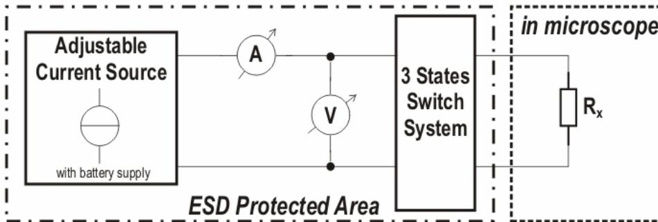
Fig. 3. Schematic presentation of the measuring circuit used for the in-situ, ground free resistance measurements
