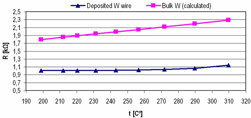
Fig. 7. Measured resistance during heat-up of the deposited wire (triangles) and the evolution expected for bulk W (squares), assuming the same room temperature resistance value for both the bulk W and the deposited wire
