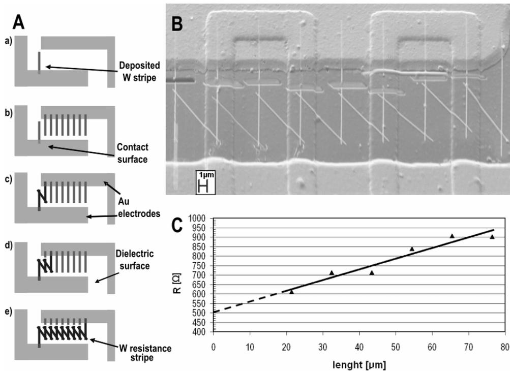
Fig. 4. Schematic presentation of the sample preparation steps for contact resistance measurement (A), illustrated on a SEM image (B), the resistance as a function of deposited wire length (C)
