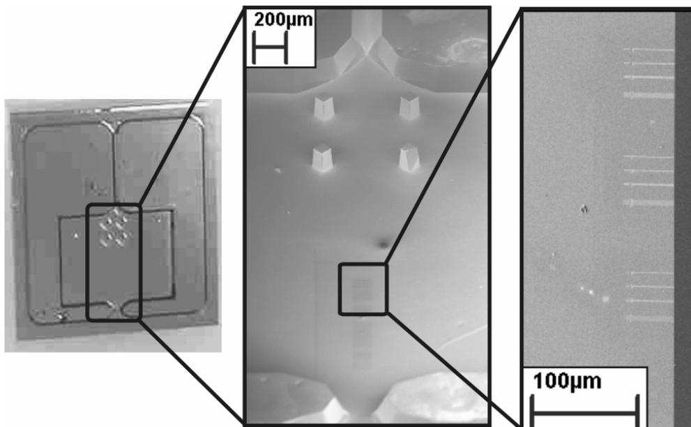
Fig. 1. Overview (left), general view with the deposition area and (middle) cleaved cross section (right) of the special cleavage sample used for the study of stripe cross-sections in the SEM
