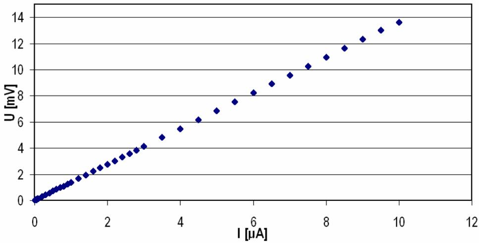
Fig. 6. The I (V) curve of a single W wire with 300 nm width
