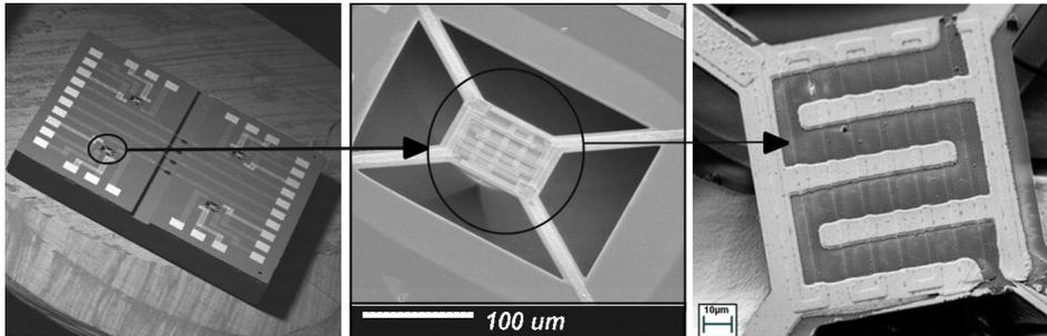
Fig. 2. The special micro-hotplate used for electrical characterisation of deposited W wires
