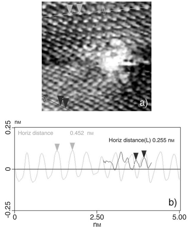
Fig. 4.  $\sqrt{3}R \times \sqrt{3}R$  – type superstructures observed near the defect in (a). The cross sectional lines in (b) show the period determined by the atomic structure (black line) and the period of the superstructure (grey line).
