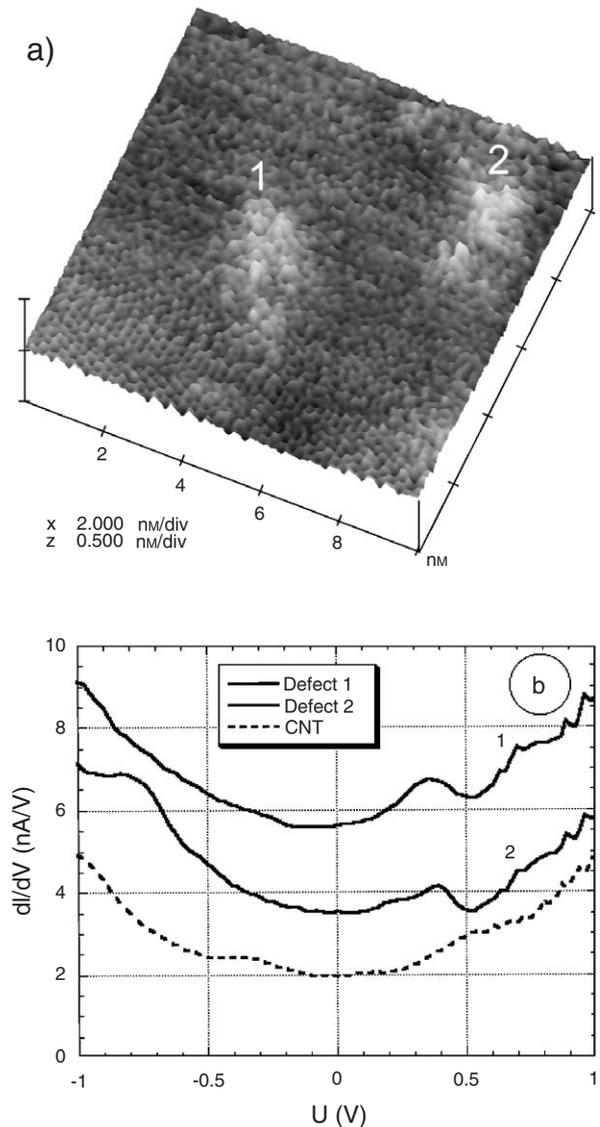
Fig. 2. (a) STM image of two nanotube defects recorded after the annealing of the irradiated sample. (b)  $dI/dV$  curves measured above the defects 1 and 2, respectively.
