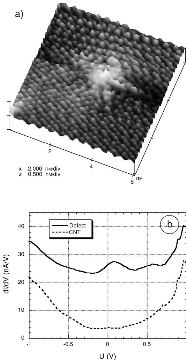
Fig. 1. (a) Atomic resolution STM image of a carbon nanotube defect produced by irradiation. (b) STS curves measured above the defect site (solid line) and above a defect-free portion of the nanotube (dashed line).
