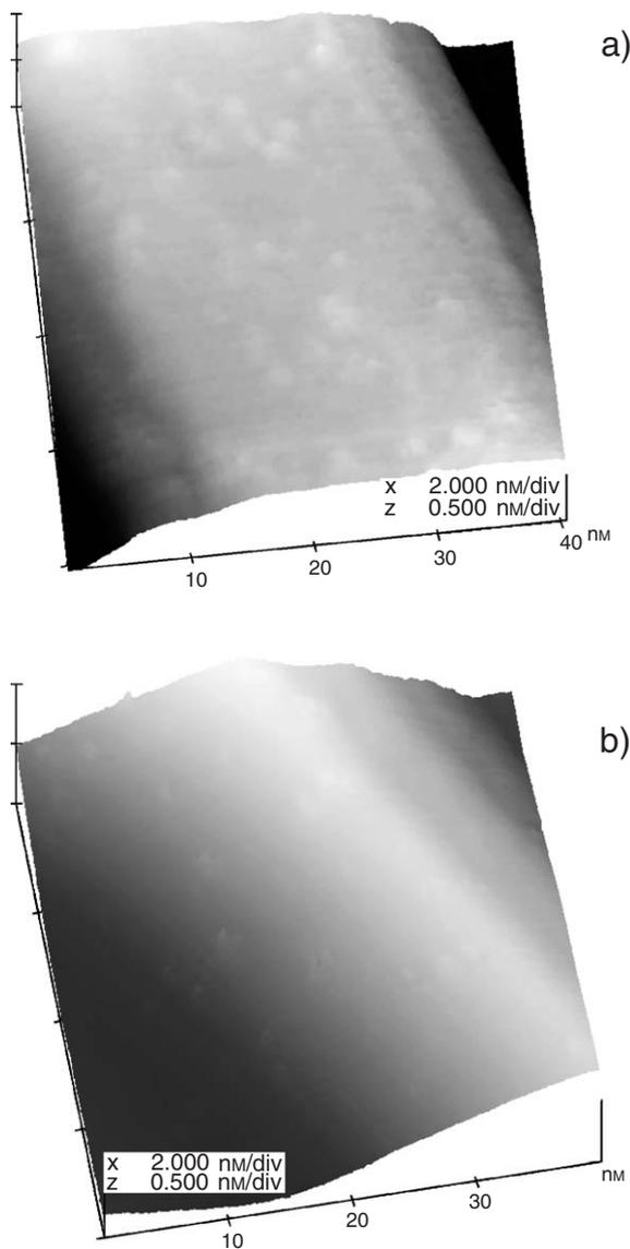
Fig. 3. 3D STM images of MWCNTs with irradiation-induced defects before (a) and after (b) annealing. After annealing the “heights” of the defects decrease.
