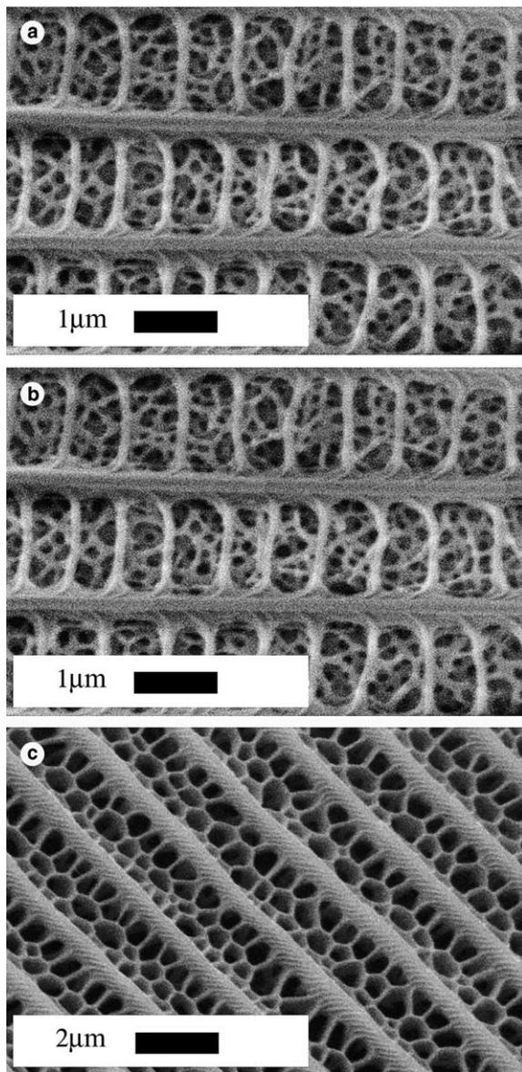
Fig. 2. SEM images showing the nanostructure of blue colored butterfly wing scales: (a) blue violet male (*Polyommatus icarus*); (b) blue male (*Polyommatus bellargus*) and (c) *Papilio ulysses*.
