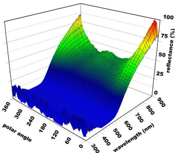
Fig. 6. Reflectance values at normal incidence natural solar illumination with reflected light picked up at  $45^\circ$  from the wing plane versus wavelength and polar angle value (the rotation axis is normal to the wing plane) for *Lycaena virgaureae* male.
