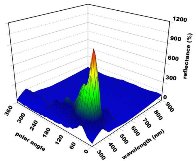
Fig. 5. Reflectance values at normal incidence natural solar illumination with reflected light picked up at  $45^\circ$  from the wing plane versus wavelength and polar angle value (the rotation axis is normal to the wing plane) for *Morpho aega* male.
