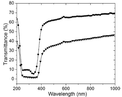
Fig. 10. Transmittance of the filament extract in ethanol: concentrated (heavy circles); after dilution (heavy triangles). One may remark that in the range below 400 nm, where the UV absorber pigment is active, the dilution had a much weaker effect than in the visible range.
