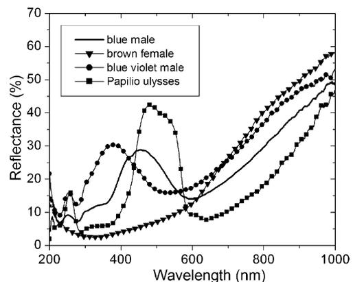
Fig. 1. Normal incidence reflectance spectra of three blue butterfly wings of different hue. The reflectance of a brown female of the same species as the blue violet male was included for comparison.
