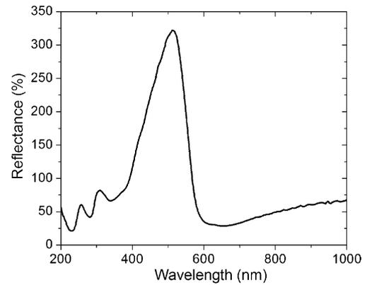
Fig. 4. Normal incidence reflectance spectra of blue *Morpho aega* male wing. The reflectance values higher than 100% are produced by the higher reflectance of the sample in a certain wavelength range than the reflectance of the white calibration standard.
