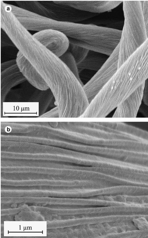
Fig. 8. SEM images of the white filamentary wool: (a) low magnification image of entangled fibers and (b) high magnification image showing the nano-relief responsible for the selective coupling of the UV light.
