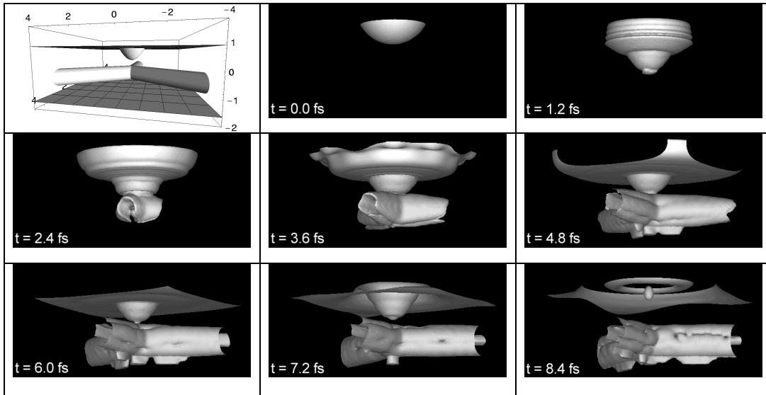
**FIGURE 1.** Time evolution of the probability density of the wave packet approaching the STM junction from the tip bulk and tunneling through the nanotube into the support. The upper left image is the model system used in the calculation. The labeled box is the presentation box. All dimensions are in  $\text{nm}$ . The subsequent images show snapshots of a constant probability density surface. This surface is clipped at the presentation box boundaries. See the text for details.
