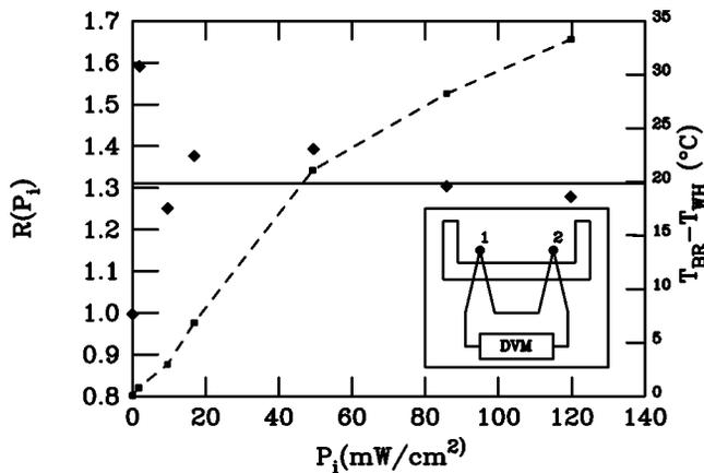
FIG. 5.  $R(P_i)$  as measured with unfiltered, artificial light from the fiber-optic illuminator as a function of incident light power density. The temperature difference between the brown (BR) butterfly and white paper is shown on the secondary axis. The inset schematically shows the setup used for the measurement.
