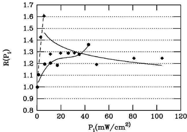
FIG. 7.  $R(P_i)$  values for yellow (diamonds) and blue (heavy circles) light illumination, using the colored glass filters. Note that the blue illumination does not produce a maximum in the range of available light power densities.
