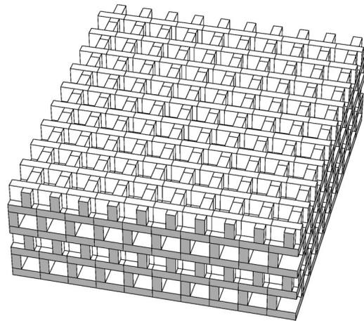
FIG. 8. Model structure built on the basis of high-resolution SEM images used in the computer simulation of the photonic crystal. The periodic structure is made of two identical layers, each  $0.2 \mu\text{m}$  thick. All chitin walls (dielectric constant  $2.25 + 0.1i$ ) are assumed to have a mean thickness of  $0.066 \mu\text{m}$ . The lateral unit cell is rectangular,  $0.24 \mu\text{m}$  by  $0.2 \mu\text{m}$ .
