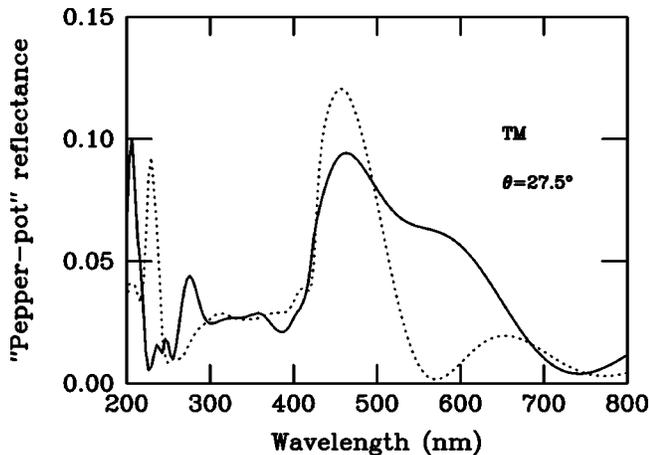
FIG. 9. Reflectance values (solid line) of the pepper-pot structure as calculated from the computer model (see Fig. 8), to be correlated with the measurements described in Fig. 3. The dotted line refers to a second, independent model, where parallelepipedic cavities are replaced by ellipsoids.
