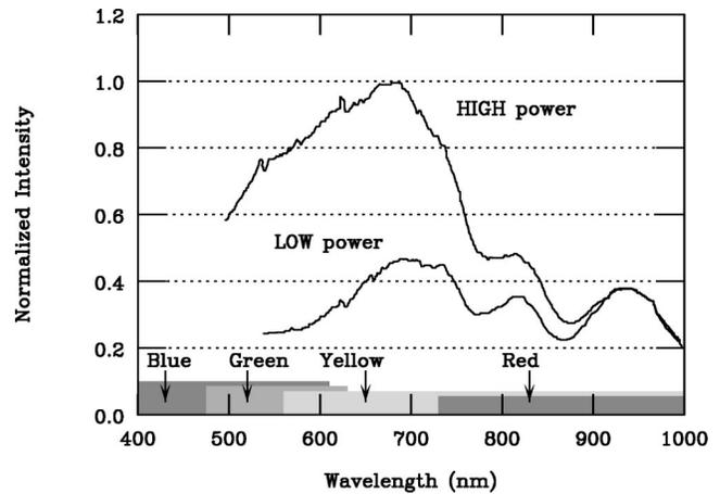
FIG. 6. Spectral distribution of the light from the fiber-optic illuminator at the lowest and the highest illumination intensities. The spectral regions in which the colored glass filters have a transmission higher than 50% are indicated.
