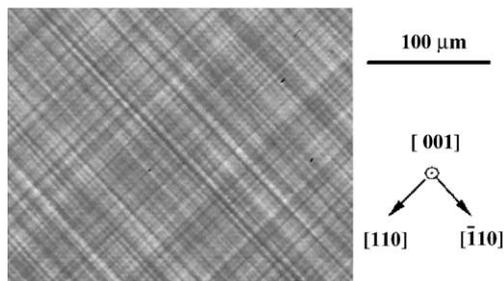
Fig. 1. Distribution of misfit dislocations at the interface of  $n^+ - p$  GaAs/ $\text{In}_{0.02}\text{Ga}_{0.98}\text{As}$  heterojunction revealed by means of EBIC technique in a scanning electron microscope.
