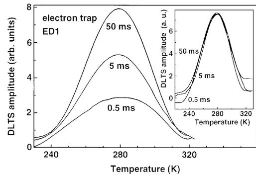
Fig. 4. DLTS line for the ED1 trap and its dependence on filling-pulse duration, whose values are written in the figure, measured at a rate window of  $2 \text{ s}^{-1}$ . In the inset, the line amplitude is normalized to the same height.
