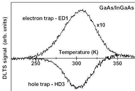
Fig. 2. DLTS spectra measured at a rate window of  $48 \text{ s}^{-1}$  for the  $n^+ - p$  GaAs/InGaAs heterojunction. The upper spectrum was recorded under reverse-bias conditions while the lower one was detected under forward-bias injection. Note the scale expansion for the upper spectrum.
