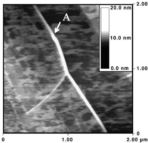
Fig. 1. AFM image of a Y-branched carbon nanotube on HOPG surface.
