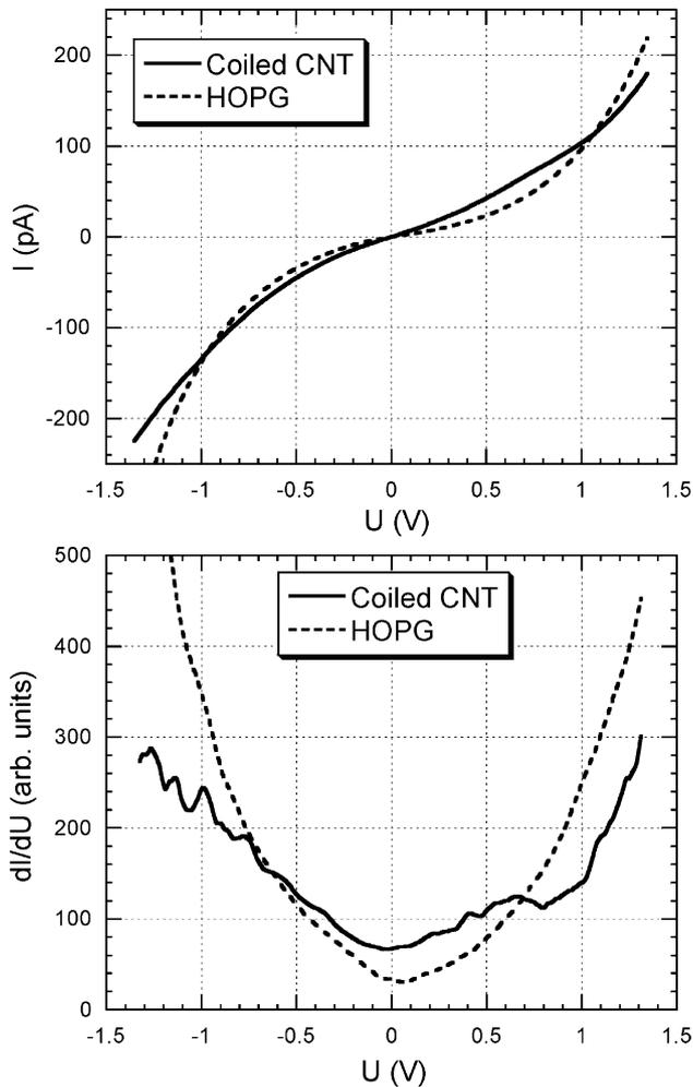
Fig. 5. Scanning tunneling spectroscopy (STS) on the coiled nanotube presented in Fig. 2a.
