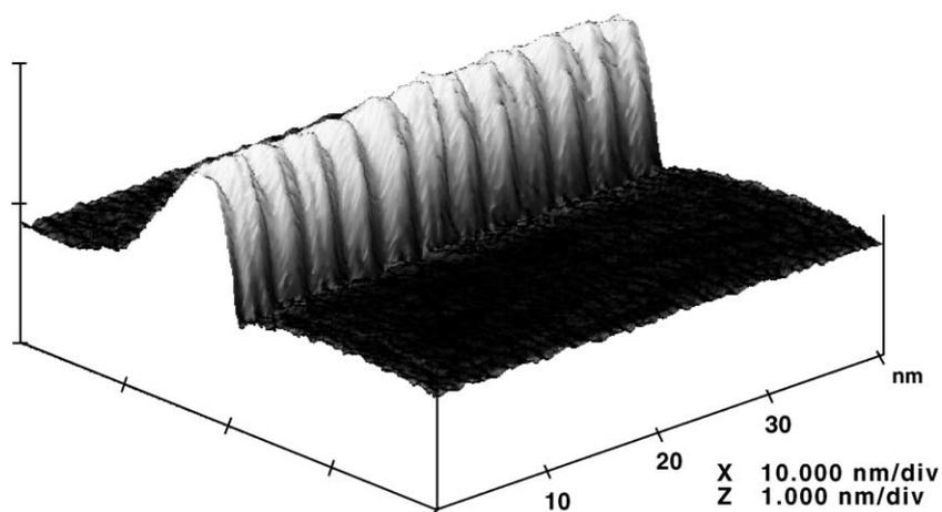
Fig. 3. Constant current topographic STM image of a coiled carbon nanotube in 3D presentation ( $I_t=200$  pA,  $U_t=1$  V).
