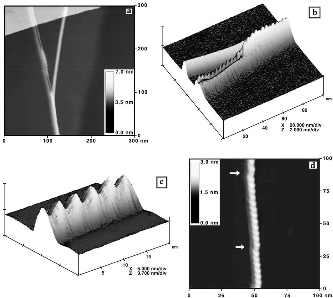
Fig. 2. Constant current topographic STM images of a coiled carbon nanotube over an Y-branched nanotube ( $I_t = 200$  pA,  $U_t = 1$  V). (a) Top view image of the coiled and the Y-branched nanotubes, both traversing a cleavage step on HOPG. (b) Higher resolution 3D representation of nanotubes. (c and d) The coiled nanotube presented in (a) at a distance of 300 nm from the place where the first image was made.
