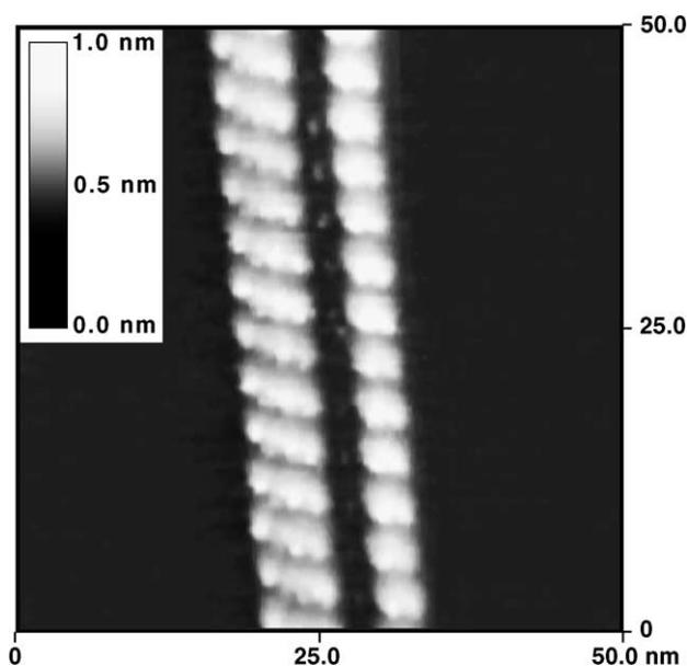
Fig. 4. Top view, constant current topographic STM image of a coiled carbon nanotube imaged with a multiple STM tip ( $I_t=200$  pA,  $U_t=1$  V).
