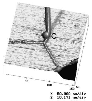
Fig. 3. Constant current topographic STM image in 3D presentation showing a Y-branched carbon nanotube, which continues with a 150° knee ( $I_{\rm t} = 250$  pA,  $U_{\rm t} = 400$  mV, PtIr tip).
