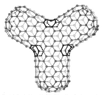
Fig. 1. Ball and stick model of the Y-branching of carbon nanotubes proposed by Scuseria [4]. Heavy line marks the six heptagons. (used with permission from Scuseria).
