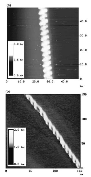
Fig. 5. Top view, constant current, topographic STM images of carbon nanotube coils: (a) tightly wound coil grown by fullerene decomposition ( $I_t = 300$  pA,  $U_t = 400$  mV, PtIr tip); (b) intercoiled tubes grown catalytically and subjected to several steps of chemical treatment ( $I_t = 150$  pA,  $U_t = 1$  V, PtIr tip).
