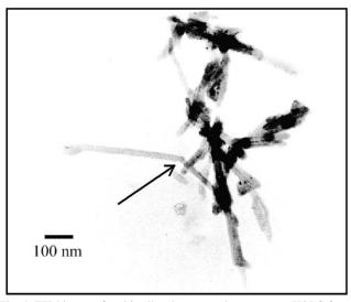
Fig. 4. TEM image of multiwall carbon nanotubes grown on HOPG from the decomposition products of  $C_{60}$ . A nanotube "knee" is marked by an arrow.
