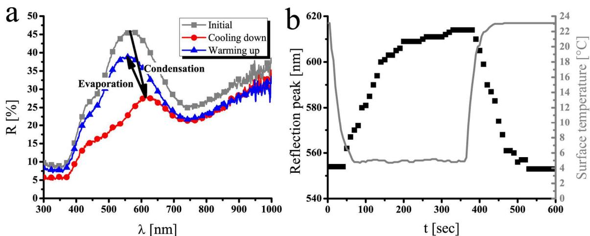
**Figure 2.** a) Change of the reflection spectrum during cooling on the green (ventral) side of *A. metallica* butterfly. b) The change of the surface temperature (gray, continuous line) and the position of the reflection maximum (black, dotted line) during cooling.
