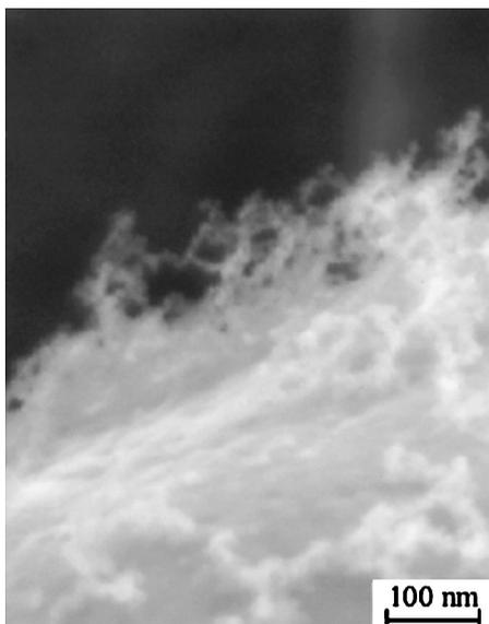
FIG. 6. SEM micrograph showing a fine nanoscale structure of a tilted molybdenum sample. A 3D structure of nanoaggregates resembles the fractal DLA and CCA clusters. Notice that large clusters and particulates are not present in this case.
